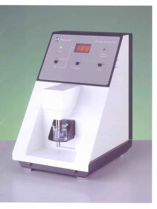
The Sherwood Model 926 is used for the determination of chloride ions. It is an instrumental analogue of "Argentimetry", the traditional titrimetric methods using silver nitrate reagent. Like these classic methods it relies on the chemical formation of the very insoluble salt, silver chloride.
